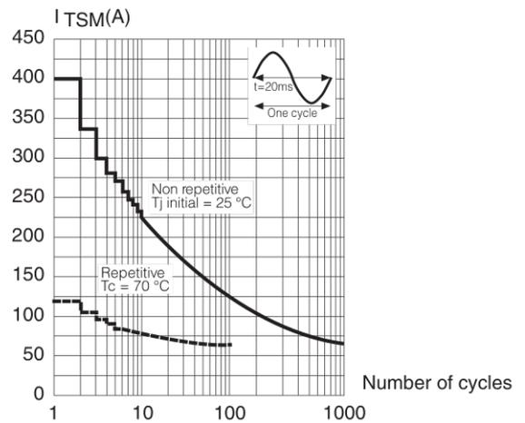
Fig. 5: Non repetitive surge peak on-state current for a sinusoidal current with width:  $t_p < 10$  ms, and corresponding value of  $I^2t$ .
