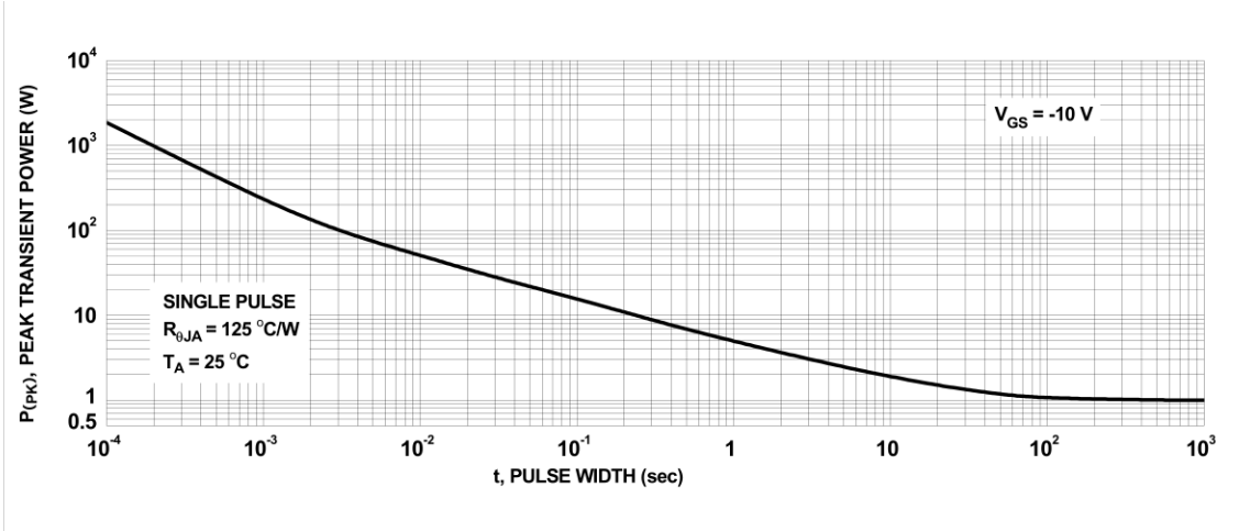
Figure 13. Single Pulse Maximum Power Dissipation
