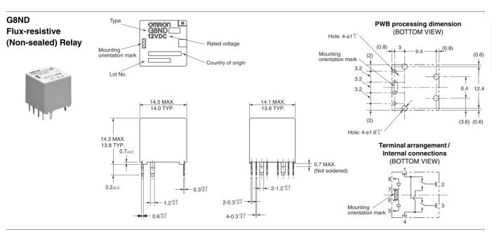
\* Tolerance unless otherwise specified Less than 1 mm: ±0.1 mm Less than 1 to 3 mm: ±0.2 mm
