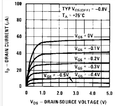
Figure 8. Common Drain-Source
