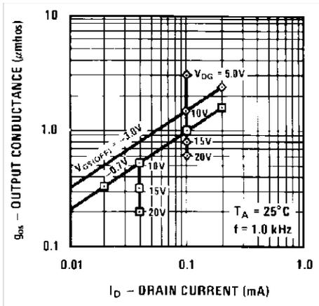
Figure 9. Output Conductance vs. Drain Current
