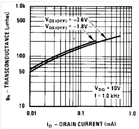
Figure 11. Transconductance vs. Drain Current
