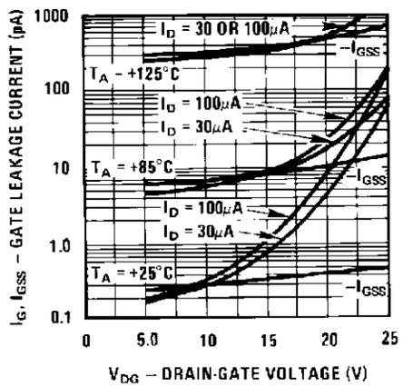
Figure 7. Leakage Current vs. Voltage
