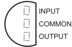
Figure 5-2. LP Package, 3-Pin TO-92 (Top View)
